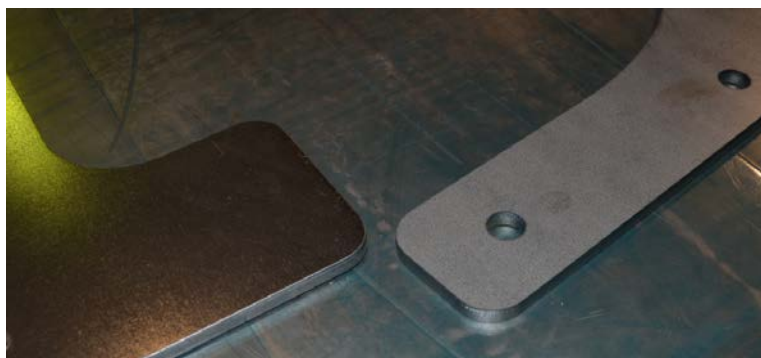
A work piece before rounding (right) and after (left).
