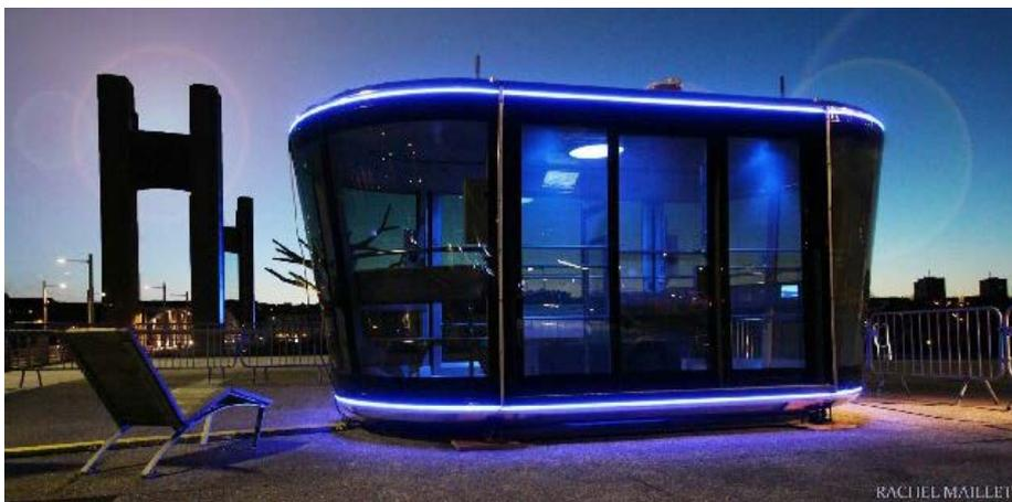
The cabins have a capacity of 60 people. They are connected to the suspension and traction cables by separate lower suspension lines, like on Funitel lifts. Constructed by Gangloff Cabins (BMF Group), they are extremely spacious and bright. They have integrated lighting and sound systems.
